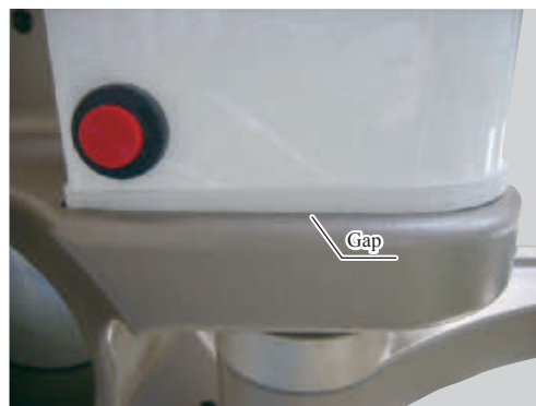
Gap at bottom of cover
